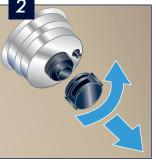
Remove steel filter cup from the steel filter holder.
